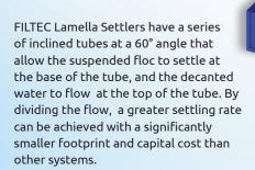
Filtration Technology have several proven FILTEC Lamella Settler designs. The vessels are fabricated from epoxy coated mild steel. They come with flow distribution at the inlet, sludge extraction devices and stainless steel launders.
