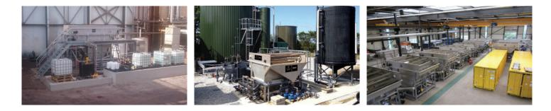
The intelligent Dissolved Air Flotation (i-DAF) system is based on the Nijhuis innovative and intelligent aeration system (i-AIRATION) which forms fine air bubbles that support and increase the separation of particles. For decades the Nijhuis Dissolved Air flotation unit has been known as the most robust and best DAF unit available on the market. The compact i-DAF with plate packs, type IPF, can either be integrated in a total solution or offered as a single product for your wastewater.
