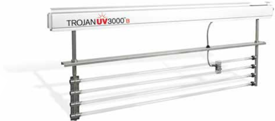
The advanced, self-contained modules incorporate convection-cooled ballasts and feature a UV lamp status indicator (below) for at-a-glance confirmation that all lamps are operating.
