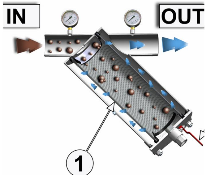
**SIMPLEX** are manual cleaning screen filters with stainless steel body, available in three building configuration: Y, L and O.
