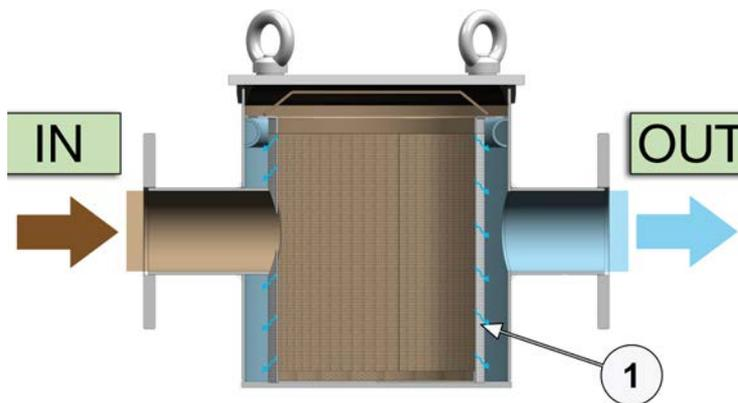
**MINI BASKET** is a manual cleaning screen filter, with stainless steel body, operating through a filtering basket in AISI 316 stainless steel which is easy to access thanks to the lid with folding closures allowing a quick and easy maintenance with reduced plant downtime.
